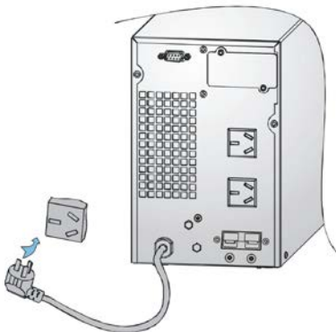
Figure 3-1 Connection Method of Input
